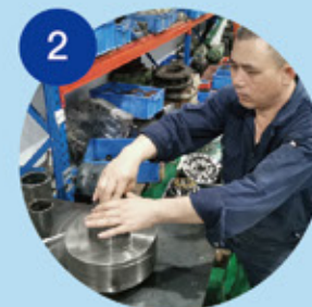
2 备件研磨修复 Cylinder Grind
